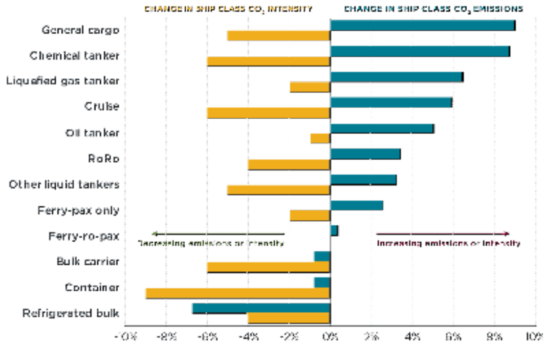
Figure E5-4. Change in CO 2 emissions and CO 2 Intensity for key ship classes
